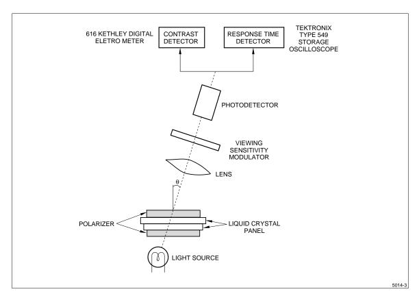
Figure 4. Optical Characteristics Test Method
