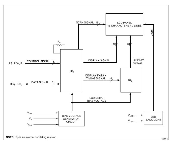
Figure 1. LM16X12A Block Diagram
