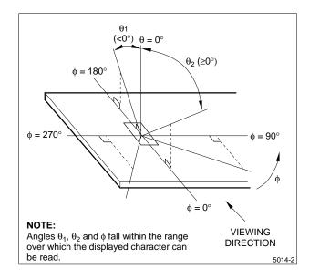
Figure 3. Definition of Viewing Angle
